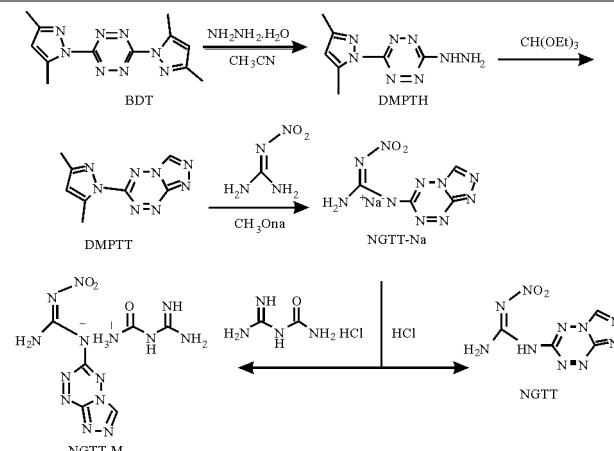
3-Nitroguanidino-1,2,4-triazolo[4,3-b]-s-tetrazine (NGTT) was synthesized and its N-guanylurea salt was obtained . Their structures , thermal stabilities , detonation velocities , detonation pressures and specific impulses as monopropellant were characterized and calculated .
