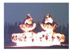
The blast power field of two-point charge at different array distances was simulated by AUTODYN software. The influence of the array distance on the explosive shock wave power of two charges was analyzed. The overpressure action area gain of two-point array charge was studied. And the relationship between the overpressure action area gain and the distance of two charges was obtained.
