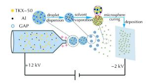
TKX-50/Al/GAP composite microspheres were prepared by electrostatic spraying . The morphology , structure and thermal decomposition properties of the microspheres were studied by SEM , XRD , FT-IR and DSC . The mechanical sensitivities of the microspheres were also tested .
