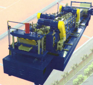
● 扇形直立缝板型自动成型机 Auto Taper Forming Machine For Standing Seam Profile
