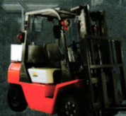
CPCDB50 防爆柴油机平衡重式叉车 CPCDB50 Explosion Diesel Forklift Trucks
