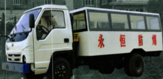
WC20R 防爆柴油机无轨胶轮车 WC20R explosion-proof rubber tire trolley car diesel engine
