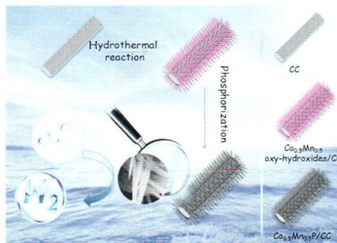
Self-supported ternary  $\text{Co}_{0.5}\text{Mn}_{0.5}\text{P}$ /carbon cloth (CC) nanomaterial was prepared through hydrothermal reaction and phosphorization process. The excellent hydrogen evolution reaction (HER) performance may derive from the synergistic effect between Co and Mn atoms and the special relative atom ratio of 1:1 from Co:Mn.
