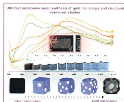
A novel, ultra-fast, simple, and highly convenient method for large scale production of the gold nanocages using microwave heating is demonstrated. Structural maneuver and atomic dislocation studies were demonstrated using electron microscopy.
