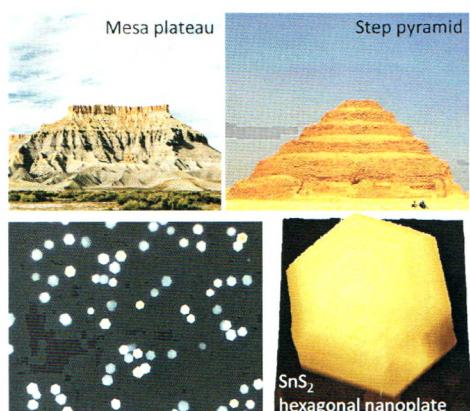
We demonstrate the controlled growth of two-dimensional (2D) hexagonal tin disulfide (SnS<sub>2</sub>) nanoflakes with stacked monolayer atomic steps.
