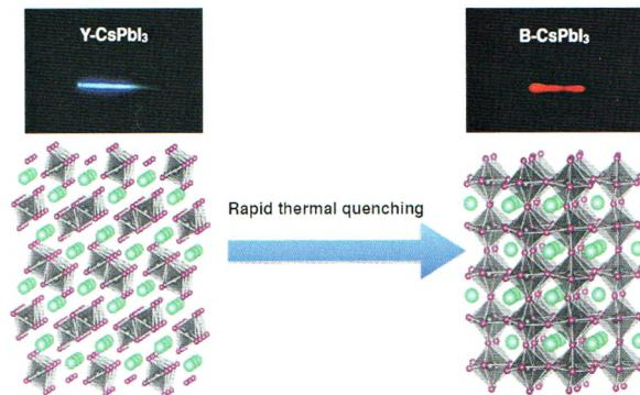
CsPbI<sub>3</sub> nanowires undergo a structural phase transition from the yellow non-perovskite phase to the black perovskite phase during rapid thermal quenching. Perovskite phase CsPbI<sub>3</sub> nanowires exhibited good optoelectronic properties for photovoltaic applications.
