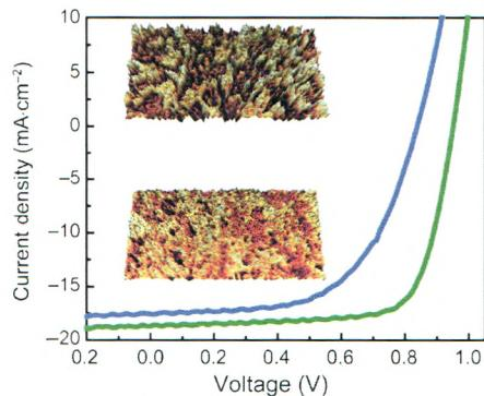
The moisture-enabled phase transition of a precursor intermediate to the perovskite phase for enhancing the photovoltaic efficiency is demonstrated. The moisture assists in decoupling the conversion and grain growth to enable the formation of active-layer films with a low defect density.
