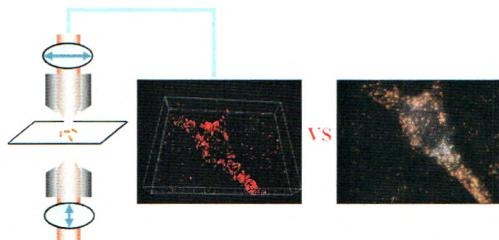
Three-dimensional plasmonic imaging of the gold-nanorod distribution inside cells with a high resolution and high contrast was achieved via orientation-dependent localization microscopy.
