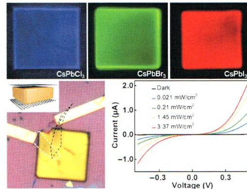
A chemical vapor deposition approach is used to grow all-inorganic cesium lead halide perovskite microplatelets and heterostructures with tunable optical and electronic properties for optoelectronic applications.
