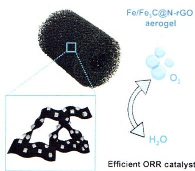
We report the rational design of a catalyst for the oxygen reduction reaction with highly active catalytic centers and enhanced active site accessibility. The catalyst was obtained via a facile Prussian blue nanoparticle approach and displayed outstanding catalytic activity on par with the state-of-the-art Pt/C catalyst at the same mass loading in alkaline media, good performance in acidic media, and excellent stability and crossover tolerance.
