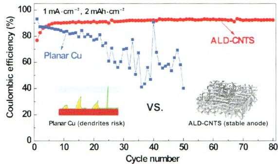
The stability of Li@atomic layer deposition (ALD)-carbon nanotube sponge (CNTS) electrodes relies on both the high-surface-area conductive framework and the robust ALD-Al<sub>2</sub>O<sub>3</sub> surface protection layer, which decreases the effective areal current density and stabilizes the electrode/electrolyte interface for Li nuclei, respectively.
