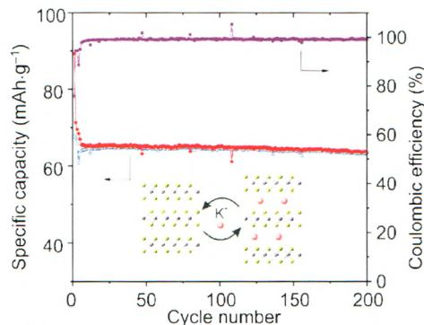
The electrochemical K<sup>+</sup> intercalation process in MoS<sub>2</sub> is shown in this study. MoS<sub>2</sub> has a long life for repetitive K<sup>+</sup> intercalation and de-intercalation.
