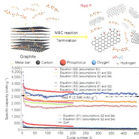
Ball-milling graphite in the presence of red P was demonstrated to produce a series of P-C composites. The capacity contributions from P and C in the P-C composites were discussed.
