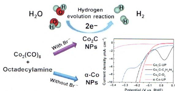
We developed a bromide-induced wet-chemistry synthesis method for Co<sub>2</sub>C nanoparticles, which were a highly active and stable electrocatalyst for the hydrogen evolution reaction.
