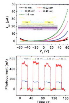
This article demonstrates the significant enhancement in the optoelectronic performance of WSe<sub>2</sub> phototransistors, via *in situ* surface functionalization with cesium carbonate. The electron mobility of WSe<sub>2</sub> was increased by nearly one order of magnitude, while the photoresponsivity and the external quantum efficiency (EQE) were enhanced by almost three orders of magnitude after Cs<sub>2</sub>CO<sub>3</sub> modification.
