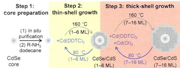
An optimized, systematic synthetic scheme for fabricating zinc-blende CdSe/CdS core/shell nanocrystals with thick shells was successfully developed.
