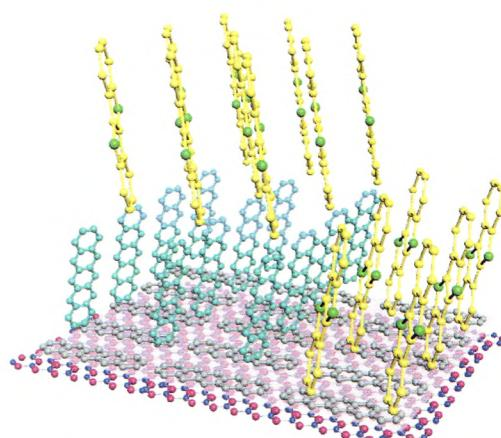
Using dioctylbenzothienobenzothiophene (C<sub>8</sub>-BTBT) and pentacene as building blocks, two-dimensional vertical and lateral molecular van der Waals heterojunctions with clean and sharp interfaces are prepared via a highly controllable physical vapor transport (PVT) process.
