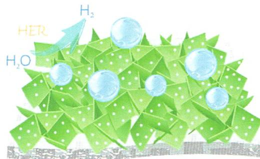
Defect-rich molybdenum disulfide nanowall electrocatalysts were successfully fabricated and exhibited robust and efficient performance in the hydrogen evolution reaction.
