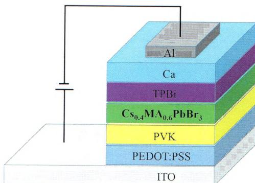
Partially replacing the organic methylammonium cations by inorganic Cs<sup>+</sup> results in perovskite thin films that provide nearly full surface coverage and much higher photoluminescence quantum efficiency due to the greater radiative recombination rate and the smaller nonradiative recombination rate. These films are therefore ideal for electroluminescence applications.
