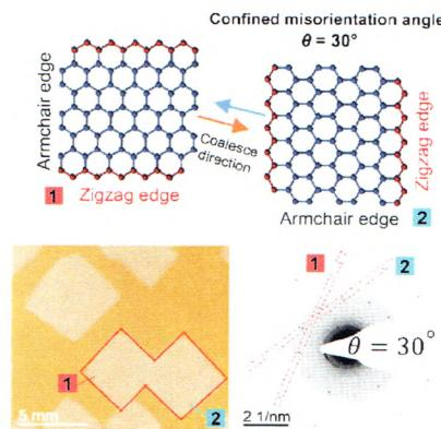
We develop a facile graphene-misorientation strategy to obtain angle-confined graphene bicrystals that contain only two lattice orientations with a tilt angle of 30°. The size of each graphene domain before coalescence is tuned from sub-centimeter (6 mm) to micrometer size using an efficient cooperative passivation strategy with a high growth rate.
