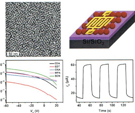
A unique PbS structure with necking percolative superlattices was used to study the effects of ligands on the electronic and optoelectronic properties of nanocrystal (NC) solids in order to elucidate the relationship between the NC surface and the properties.
