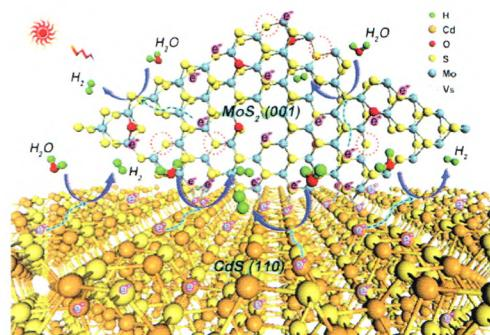
Without using noble metals as co-catalysts, multi-node CdS hetero-nanowires (NWs) were grown with defect-rich O-incorporated MoS<sub>2</sub> ultrathin nanosheets (NSs). The hetero-NWs exhibited abundant catalytic active sites, substantially improved electric conductivity, and significantly enhanced separation of charge carriers, resulting in superior visible-light photocatalytic properties compared with Pt/CdS NWs, pure CdS NWs, and MoS<sub>2</sub> NSs, as well as their physical mixtures.
