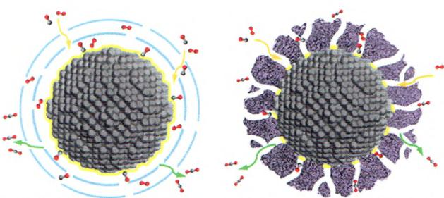
Pt@hexagonal boron nitride (h-BN) core–shell nanostructures function as nanoreactors, in which CO oxidation reactions with improved activity, selectivity, and stability occur at the core–shell interfaces. The confinement effect exerted by the h-BN shells promotes the Pt-catalyzed reactions.
