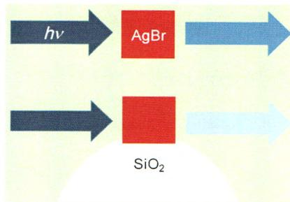
An increased absorption cross section in semiconductor AgBr nanoparticles is achieved by placing them on dielectric SiO<sub>2</sub> nanospheres that generate enhanced scattering nearfields.
