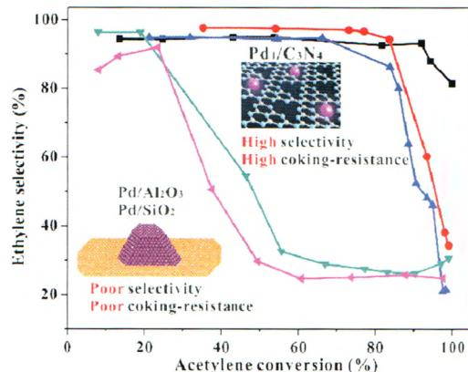
A single-atom Pd<sub>1</sub>/C<sub>3</sub>N<sub>4</sub> catalyst showed a remarkably high ethylene selectivity and excellent durability by effectively suppressing coke formation during selective hydrogenation of acetylene in excess ethylene.
