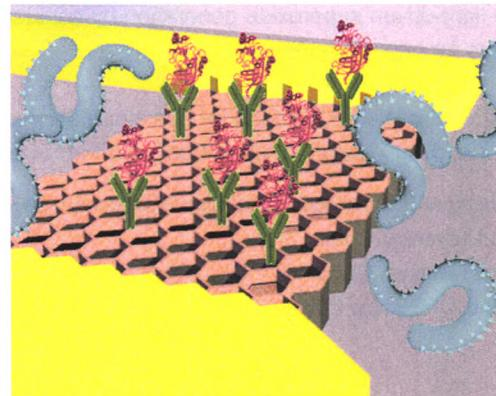
We demonstrate the biosensing of the Ebola VP40 matrix protein in liquid samples, using a memristor mode of a nanodevice. Further, we show the advantages of controlling the voltage gap via external voltage, which allows the sensing of both positive and negative charges.
