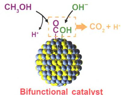
Using surface controlled PtNi alloy nanoparticles as model catalysts, we propose that the methanol oxidation reaction (MOR) undergoes a Langmuir–Hinshelwood mechanism. Bifunctional catalysts with both CO and OH adsorption sites are beneficial for promoting the MOR in an alkaline electrolyte.
