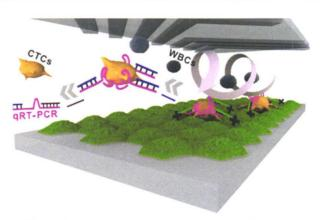
In this study, we developed a programmable DNA-responsive microchip integrated with a hierarchical nanostructure for highly efficient capture, nondestructive release, and detection of protein biomarkers of circulating tumor cells.
