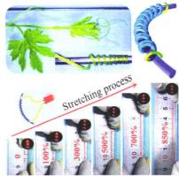
An ultra-stretchable wire-shaped supercapacitor was fabricated by winding fibrous electrodes around an elastic core fiber. The supercapacitor can sustain tensile strain up to 850%, while maintaining a stable electrochemical performance. This study provides a universal strategy for the fabrication of highly stretchable wire-shaped devices.
