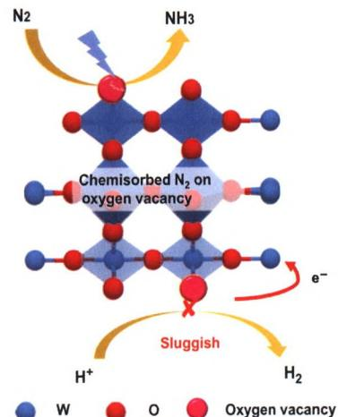
The  $\text{WO}_3$  nanosheets with oxygen vacancy were designed for nitrogen reduction reaction (NRR) and tuned electroinc state to suppress hydrogen evolution reaction (HER).
