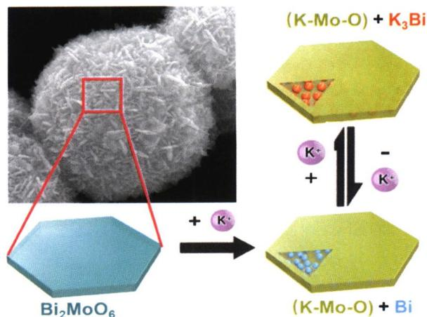
$\text{Bi}_2\text{MoO}_6$  microsphere assembled by two-dimensional (2D) nanoplate exhibits good potassium storage performance and performs a combination mechanism of conversion reaction and alloying/dealloying reaction.
