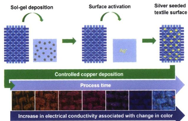
*In situ* growth and immobilization of copper nanoparticles on cellulose textiles results in tunable coloration and electrical conductivities.
