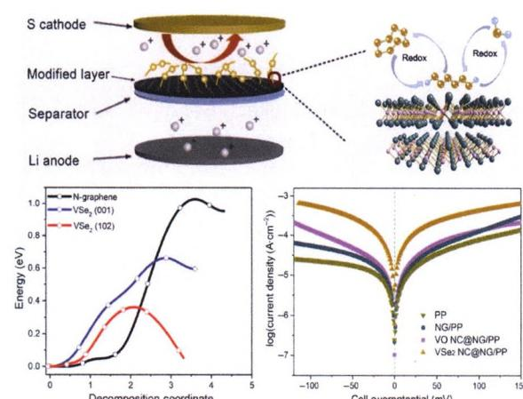
VSe<sub>2</sub> ultrafine nanocrystals immobilized on the nitrogen-doped graphene hybrid nanosheets (VSe<sub>2</sub> NC@NG) as a new polysulfides barrier are synthesized via a self-template strategy, which possess more exposed sulfophilic planes of VSe<sub>2</sub>, as well as benefit the uniform nucleation of Li<sub>2</sub>S—making this system an excellent polysulfides barrier for lithium–sulfur batteries.
