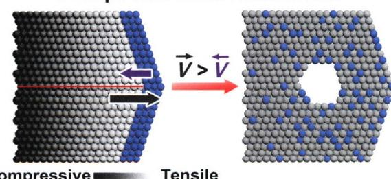
Kirkendall effect unexpectedly takes place when diffusing intrinsically faster Cu atoms into Pd icosahedra. The strain gradient arising from the multiple twins of the icosahedra is the key to drive such Kirkendall effect, leading to the formation of hollow structures.
