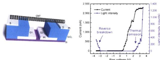
We report broadband electroluminescence via highly efficient light emission through an avalanche breakdown process from individual suspended carbon nanotube (CNT) dual-gate field effect transistor (FET) devices. The corresponding spectra obtained via thermal emission are considerably narrower than those obtained under reverse breakdown.
