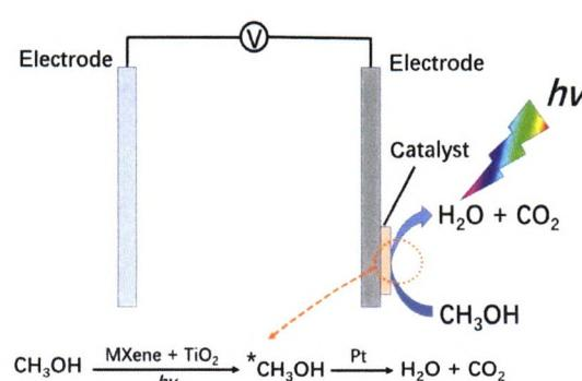
A Pt-MXene-TiO<sub>2</sub> composite exhibits highly efficient methanol oxidation reaction (MOR) performance with light irradiation via a photo-active cascaded electro-catalytic process.
