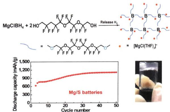
Gel-type electrolytes are advantageous in terms of safety and flexibility compared with liquid electrolytes. Here, a non-nucleophilic gel-type magnesium chloride-(fluorinated tetraethylene glycolic)borate ( $\text{MgCl-FTGB}$ ) electrolyte is synthesized. Mg deposition and stripping can be conducted with high rate and low overpotential in this electrolyte. It is also compatible with S cathode and enables stable cycling of Mg/S batteries.
