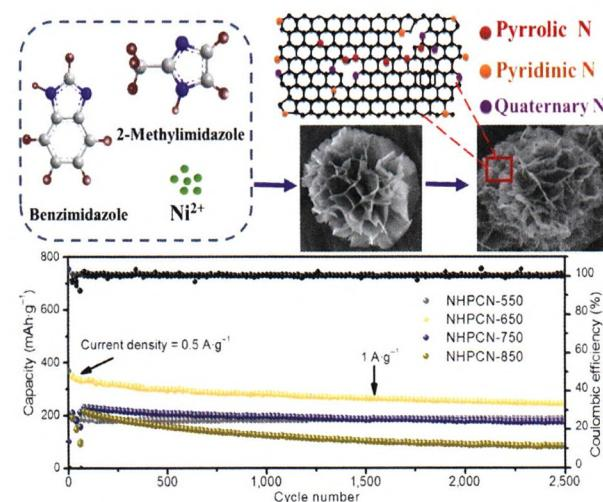
A novel self-template strategy is designed to synthesize uniform flowerlike N-doped hierarchical porous carbon networks (NHPCN) with high content of N (15.31 at.%), expanded interlayer spacing, ultrathin two-dimensional nano-sized subunits, and three-dimensional porous network structure, delivering outstanding sodium storage performances.
