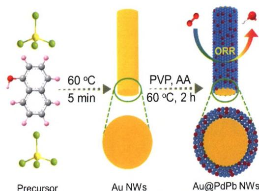
Trimetallic Au@PdPb nanowires (NWs) are synthesized by using pre-fabricated ultrathin Au nanowires as the one-dimensional template. The Au@PdPb NWs are demonstrated to be active and stable for the oxygen reduction reaction (ORR), much better than those of commercial Pd black and bimetallic Au@Pd NWs. Considering facile synthesis method and excellent ORR performance, the developed Au@PdPb NWs may have great potential in the field of fuel cells.
