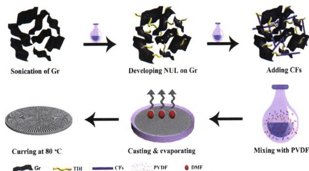
The nanourethane linkage (NUL) based graphene (Gr) and carbon fibers (CFs) 3D architecture (NUL-Gr/CFs) is fabricated, which is further employed in making composite of polyvinylidene fluoride (PVDF). Herein, toluene diisocyanate (TDI) is utilized to develop NUL.
