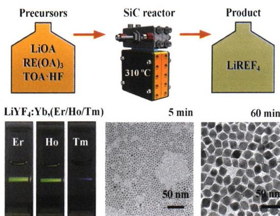
A continuous method for synthesizing  $\text{LiREF}_4$  nanocrystals was developed with the assistance of a new precursor solution and a silicon carbide (SiC) reactor. The new precursor solution employed trioctylamine (TOA) as the solvent, which prevented the generation of unnecessary solid components, and the space-time yield of the continuous method is about 15 times of that traditional batch reactions.
