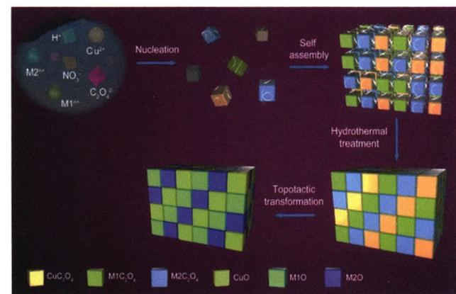
A general bottom-up synthesis of CuO-based trimetallic oxide mesocrystals (denoted as CuO-M1O<sub>x</sub>-M2O<sub>y</sub>, where M1 and M2 = Zn, In, Fe, Ni, Mn, and Co) is reported using a simple precipitation method followed by a hydrothermal treatment and a topotactic transformation via calcination.
