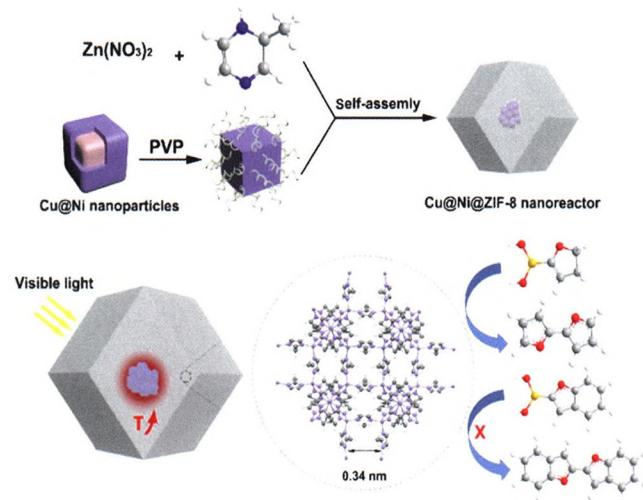
A multifunctional nanoreactor for C–C coupling reaction was successfully designed via encapsulating the core-shell Cu@Ni nanocubes into ZIF-8 (Cu@Ni@ZIF-8).
