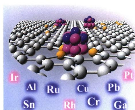
A library of ultrasmall bimetallic nanoparticles with average particle sizes ranging from 0.7 to 1.4 nm are prepared on mesoporous sulfur-doped carbon supports. The synthetic approach is based on the strong chemical interaction between the doped sulfur atoms on carbons and metals, which suppresses the metal aggregation during H<sub>2</sub>-reduction and ensures the formation of small-sized and alloyed bimetallic nanoparticles.
