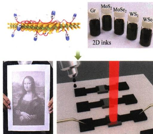
Various two-dimensional transition metal dichalcogenide (TMD) nanosheets, in addition to few-layered graphene, are inkjet-printed using a novel liquid-phase exfoliation process based on zwitterionic dispersants in water. Aqueous, biocompatible zwitterionic inks with TMD nanosheets are suitable for conventional office inkjet printing, giving rise to the mechanically flexible, printed arrays of two-terminal, parallel type photodetectors with pixelated TMD channels.
