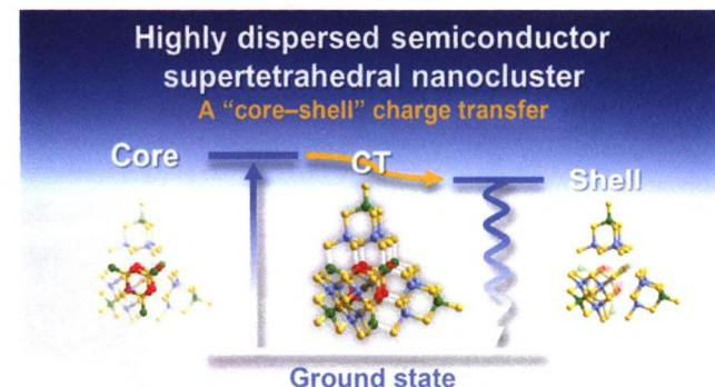
A unique “core–shell” charge transfer relaxation dynamics directed by composition variation was observed in a group of atomically precise semiconductor nanoclusters with targeted high dispersibility in solution.
