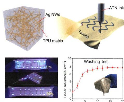
Printable elastic conductor with conductivity of  $3,668 \text{ S} \cdot \text{cm}^{-1}$  was developed for electronic textiles (e-textiles). One-step printing of ink could fabricate robust e-textiles, which could endure repeated stretching, folding, and machine washing.
