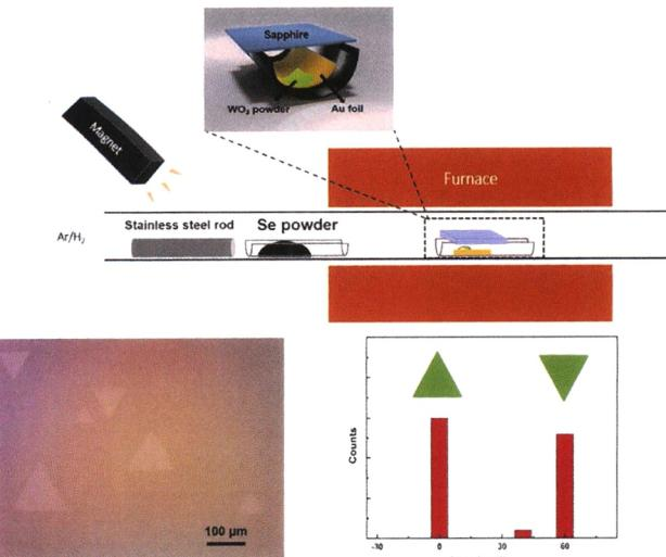
Gold vapor was introduced into the chemical vapor deposition (CVD) process as a catalyst to assist the growth of WSe<sub>2</sub>. Highly aligned monolayer WSe<sub>2</sub> triangular flakes with large domain size ( $130 \mu\text{m}$ ) and fast growth rate ( $4.3 \mu\text{m}\cdot\text{s}^{-1}$ ), and continuous monolayer films with good uniformity were achieved.
