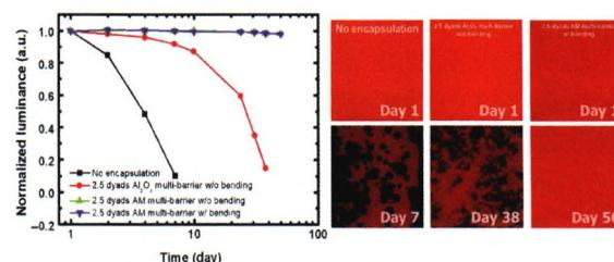
An  $\text{Al}_2\text{O}_3/\text{MgO}$  nanolaminate was fabricated and it exhibited greatly improved hydrolysis resistance in harsh environmental conditions than  $\text{Al}_2\text{O}_3$ . An actual encapsulated operating device was tested under bending stress and the device demonstrated excellently stable shelf-lifetime in a harsh environment.
