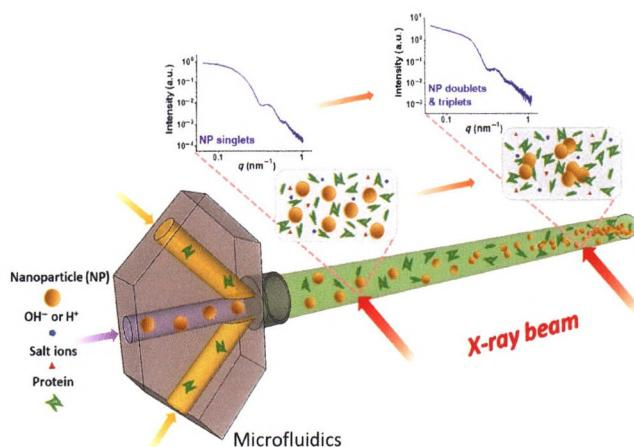
An advanced label-free method based on small-angle X-ray scattering (SAXS) and microfluidic for *in situ* measurements of dynamic processes, namely nanoparticles agglomeration in biological media is reported.
