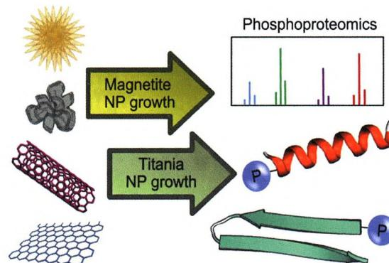
Nanocomposites are prepared from different carbon nanostructure scaffolds for magnetite and titania nanoparticle nucleation and growth. Their performance surpasses the commercial reference in NanoHPLC-MS/MS analysis of cancer cell lysates for phosphopeptide enrichment and detection.
