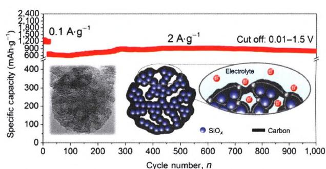
A well-engineered porous nanostructure is designed to realize the wet-chemistry preparation of a high-performance SiO<sub>x</sub>@C nanocomposite.
