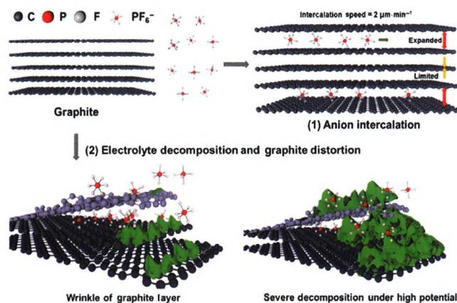
*In situ* atomic force microscope (AFM) reveals the  $\text{PF}_6^-$  anion intercalation in graphite-based dual ion batteries (DIBs) and monitors electrolyte decomposition and graphite structure evolution at nanoscale.
