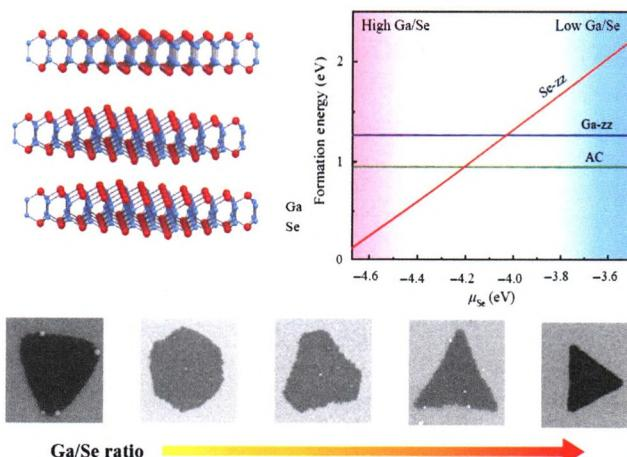
The use of gallium in precursor is demonstrated to control the shape evolution of monolayer GaSe crystals with variation from curved triangular, hexagonal to regular triangular geometries. Shape evolution behavior of GaSe flakes can be elucidate by the change of Ga/Se ratio in the precursors influence on the kinetic growth dynamics of edges.
