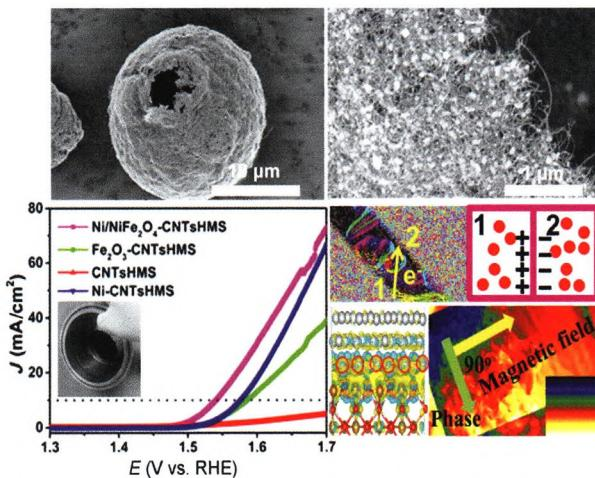
The novel nanostructure design for Ni/NiFe<sub>2</sub>O<sub>4</sub>-CNTs composite microsphere (< 14 μm) forcibly-assembled by zero-dimensional nanoparticles units (< 16 nm) and one-dimensional self-supporting CNTs has endowed the composite with enriched polarized heterojunction interface and hierachal conductive network, which thus have facilitated greatly catalytic activity and conductivity, ultimately improving the oxygen evolution reaction (OER) performance.
