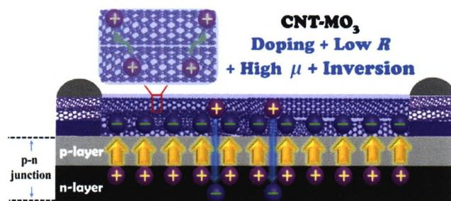
Taking advantage of transformation from transition metal chloride to oxide, the carbon nanotube (CNT)-Si solar cells have been significantly improved by p-doping effect combined with enhanced carrier mobility and inversion layer formation within Si, and achieved 16% cell efficiency based on metal chloride/oxide optimization.
