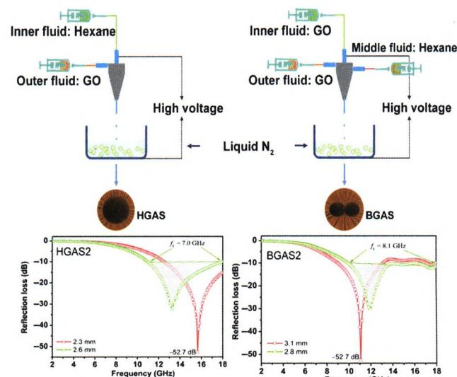
Multiaxial electrospun hierarchical hollow graphene aerogel spheres exhibit high-performance microwave absorption.
