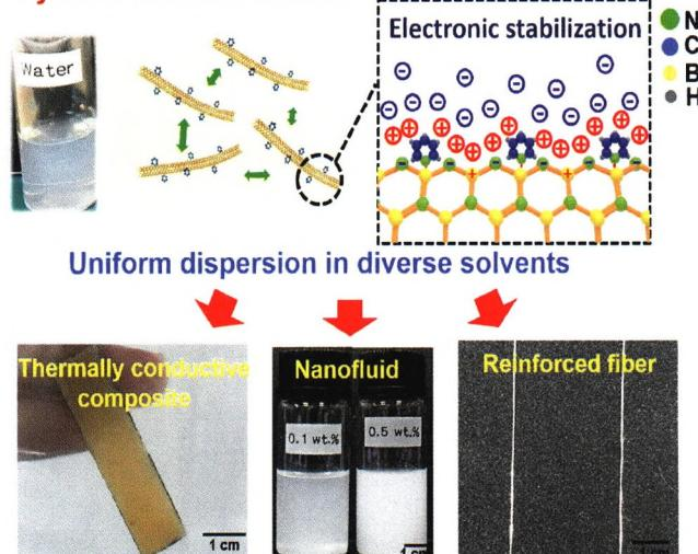
This study demonstrates the dispersion of boron nitride nanotubes (BNNTs) in diverse solvents with the use of pyridine for applications in thermally conductive composite, nanofluid, and reinforced fiber.
