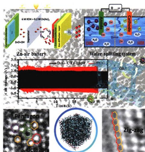
A novel boric acid-splicing and pyrolysis treatment strategy is proposed to fabricate the sponge-like unadulterated carbontube-graphene complexes (D/G-CTs) with hierarchical porous architecture as highly efficient trifunctional electrocatalysts with widespread application prospect for oxygen transformation and overall water splitting in the sustainable energy conversion techniques.
