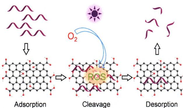
DNA oligonucleotides are first adsorbed on graphene oxide and then cleaved by the light induced reactive oxygen species followed by the desorption of short product fragments to complete a nanozyme catalytic cycle.
