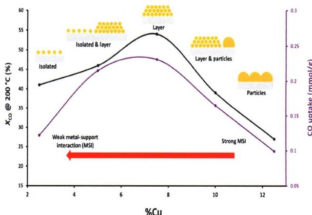
The interfaces between copper nanoparticles and one-dimensional titanium dioxide nanorods (TNRs) support can be tailored with different interfacial site activities for CO oxidation through changing the metal loading and the degree of reduction. The interfacial site activity is highly dependent on the morphology of the titanium dioxide support.
