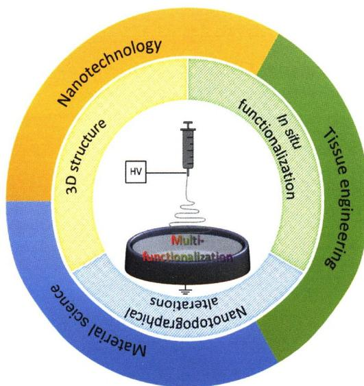
Wet electrohydrodynamics is an emerging technique that enables multi-functionalization of submicron fibers as 3D macrostructures with tunable nano-topography and homogeneous chemical modifications in one single step.
