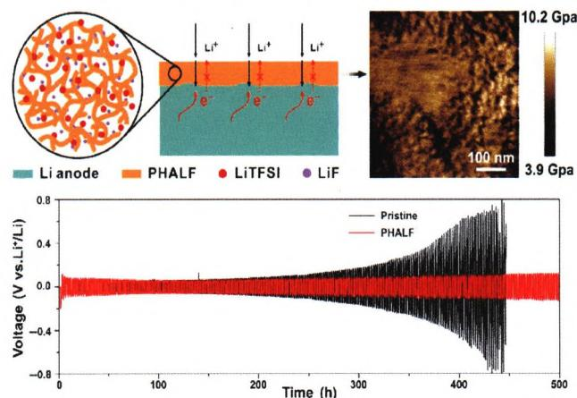
PHALF solid electrolyte interface (SEI) composed of flexible polymer substrate and inorganic LiF is constructed by one-step *in situ* photopolymerization serving as an artificial SEI, which is stiffness-enough to suppress dendrites growth and stable to protect lithium metal anodes from side reactions in high operating voltage systems.
