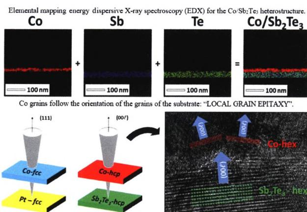
The atomic layer deposition of Co on top of Sb<sub>2</sub>Te<sub>3</sub> and Pt substrates evidences the substrate selectivity of such a deposition process, also achieving a local epitaxy and an extremely high conformality of the Co thin films.
