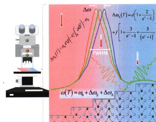
The anharmonic behaviors of phonons in WSe<sub>2</sub> flakes with different thicknesses are obtained from temperature-dependent Raman spectroscopy studies.
