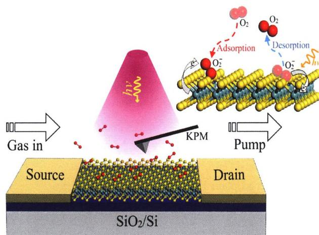
The ultraviolet (UV) illumination enhanced O<sub>2</sub> desorption on monolayer MoS<sub>2</sub> is demonstrated by electrical, optical and Kelvin probe techniques. The photo-excited charge transfer photodesorption model is proposed.
