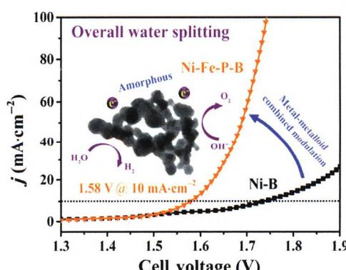
Quaternary amorphous Ni-Fe-P-B nanoparticle catalyst was synthesized by a facile, green and scalable wet-chemical reduction method. The metal-metalloid combined modulation endows Ni-Fe-P-B enhanced bifunctional activities towards both hydrogen evolution reaction (HER) and oxygen evolution reaction (OER), giving rise to considerably improved water splitting performance in comparison with binary Ni-B.
