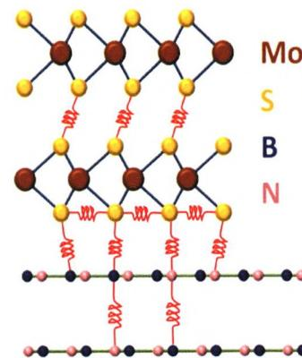
We investigated the interlayer coupling of the van der Waals (vdW) heterostructure of MoS<sub>2</sub> and hexagonal boron nitride (h-BN) over a wide range of temperatures using Raman scattering and photoluminescence.
