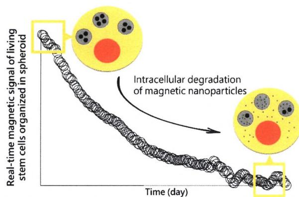
The internalization and progressive degradation of magnetic nanoparticles within stem cells is assessed at the single spheroid level, in real-time, in the biological environment, on alive samples, using a benchtop-size magnetic sensor, without impacting cell functionality.
