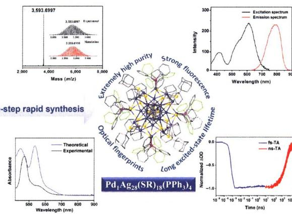
One-step rapid protocol was developed to synthesize novel Pd-doped Ag nanocluster with high yield. The prepared [Pd<sub>1</sub>Ag<sub>28</sub>(S-Adm)<sub>18</sub>(PPh<sub>3</sub>)<sub>4</sub>]<sup>2+</sup> nanocluster exhibits intriguing crystal structure, high purity, strong near infrared (NIR) fluorescence, unique optical fingerprint and unexpectedly long excited-state lifetime.
