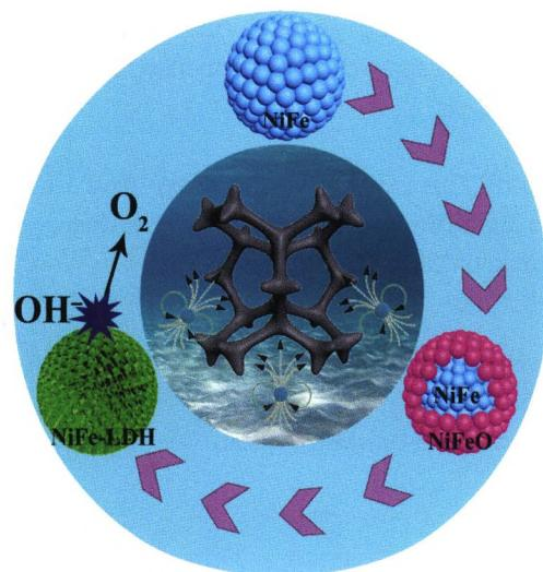
A facile self-magnetic-attracted approach was developed to construct Ni<sub>x</sub>Fe<sub>(1-x)</sub>@Ni<sub>x</sub>Fe<sub>(1-x)</sub>O/NF with excellent performance towards alkaline oxygen evolution reaction.
