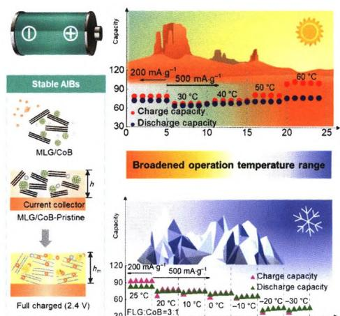
Multi-functional cobalt boride nanoclusters are employed into few-layer graphene for achieving composite positive electrode for Al batteries, which present enhanced electrochemical and mechanical stability along with broadened operation temperature range ( $-30\text{--}60\text{ }^\circ\text{C}$ ). The results suggest exclusive advantages using integrated ionic intercalation-redox reaction mechanism for designing and fabricating advanced wide-temperature Al batteries.
