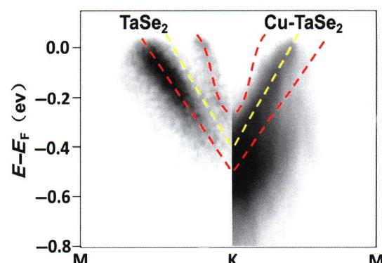
Taking advantage of X-ray absorption fine structure and angle-resolved photoemission spectroscopy, we studied how Cu intercalation influences the host TaSe<sub>2</sub> layers in Cu<sub>0.03</sub>TaSe<sub>2</sub> crystals. By examining the changes of band dispersions, we show that the variation of electronic structures is related to the bonding and charge transfer between intercalated Cu and Se atoms.
