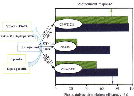
Crystal phase engineering of polytypic CuInS<sub>2</sub> (CIS) nanosheets (chalcopyrite/wurtzite and zincblende/wurtzite) was the first time achieved using oleic acid and liquid paraffin as the low-cost and environmental-friendly hot-injection system. The essential relationship between the polytypic structure and the photocatalytic/photoelectrochemical properties was lighted.
