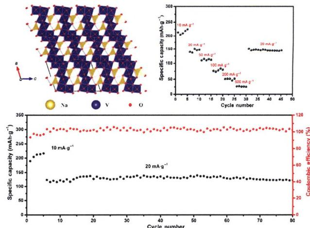
Herein, we have prepared the enlarged layer spacing  $\text{NaV}_6\text{O}_{15}$  with many vacancies for the  $\text{Mg}^{2+}$  insertion. The  $\text{NaV}_6\text{O}_{15}$  not only exhibits high discharge capacity ( $119.2 \text{ mAh}\cdot\text{g}^{-1}$  after 100 cycles at the current density of  $20 \text{ mA}\cdot\text{g}^{-1}$ ), but also expresses the good rate capability.
