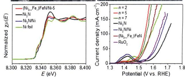
The porous hierarchical hetero- $(\text{Ni}_{3-x}\text{Fe}_x)\text{FeN}/\text{Ni}$  composites are *in situ* constructed for the efficient electrocatalytic oxygen evolution reaction (OER), and the optimized catalyst exhibits an excellent performance with a low overpotential of 223 mV@10 mA·cm<sup>-2</sup>, a small Tafel slope of 68 mV·dec<sup>-1</sup>, high Faradaic efficiency of 97.6% as well as a high stability.
