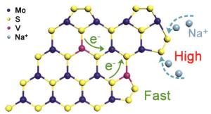
The supersaturated bridge-sulfur and vanadium co-doped  $MoS_2$  nanosheet delivers ultrahigh sodium storage capacity and fast reaction kinetics.
