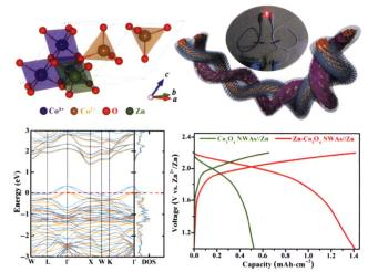
Density functional theory (DFT) calculations demonstrate that the substitution of Zn for Co<sup>3+</sup> leads to an insulator-metal transition in the Zn-doped Co<sub>3</sub>O<sub>4</sub>. High-performance fiber-shaped aqueous rechargeable Co//Zn battery with 2.2 V-high voltage based on Zn-doped Co<sub>3</sub>O<sub>4</sub> was demonstrated.
