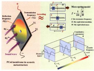
A superbroad-band actively tunable acoustic metamaterials consisting of a laminated poly (ethylene terephthalate)/carbon nanotube (PET/CNT) nanocomposite membrane were proposed, which exhibits adjustable acoustic bandwidth of 419 Hz under low applied voltage of 60 V, resulting in great potential in noise reduction applications.
