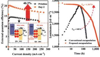
By developing a physical model and an analytical model, we identify that the positive aging of quantum-dot light-emitting diodes (QLEDs) is mainly attributed to the suppression of hole leakage current that is resulted from the passivation of ZnMgO defects. To fully take the advantage of positive aging, a new encapsulation method is proposed, which improved the device lifetime by 6.0 folds.
