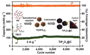
${\rm TiP_2O_7}$  as a promising Ti-based anode material, combines enhanced specific capacity, increased Coulombic efficiency and low operation voltage together. These features can be associated with the underlying electrochemical reactions for Na storage, very different from the case of  ${\rm TiO_2}$ .
