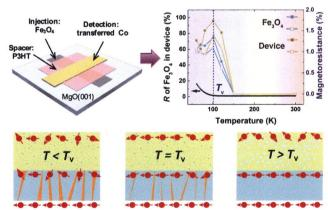
Drastic enhancement of magnetoresistance (MR) ratios was achieved at Verwey transition point in polymer spin valve with vertical configuration of  $Fe_3O_4/P3HT/Co$ .
