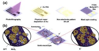
The hybrid three-dimensional stereo nanostructure, including  $MoS_2$  nanosheets and graphene fishnet tube (GFT), provides the  $K^+$  ions with a short diffusion pathway and more active sites, and the different phases of  $MoS_2$  play different roles in different devices of the multifunctional systems.
