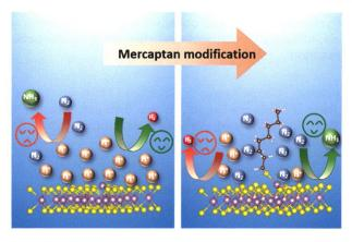
$MoS_2$  after thiol modification increased the local  $N_2$  concentration, inhibited the hydrogen reduction reaction (HER), and facilitated the adsorption of  $N_2$ , which further improved the nitrogen reduction reaction (NRR) activity.
