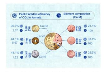
We successfully demonstrate the "third side of a coin" as an efficient CO<sub>2</sub> reduction catalyst. A closed-loop lifecycle of formate/formic acid was developed, promising as an industry-compatible commodity chemical.
