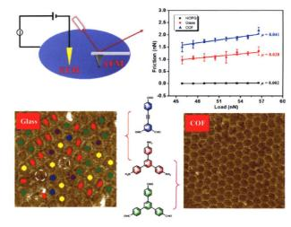
The large-scale, continuous, and low-defect glassy covalent organic networks (GCONs) was constructed based on dynamic covalent chemistry on surface, and the GCONs have lower friction coefficient in comparison with crystalline covalent organic frameworks (COFs).
