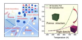
The difference in morphology of PbS nanocrystals leads to different stackings, tunable thermal conductivity. Ultimately the zT value of the porous structure (4#) is greatly improved under the multiple phonons scattering mechanism as compared to the high-density sample (5#).
