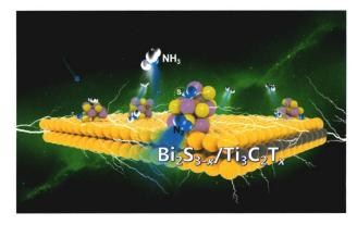
Sulfur-deficient Bi $_2$ S $_{3-x}$  nanoparticles decorated Ti $_3$ C $_2$ T $_x$ -MXene exhibited a dramatically boosted electrocatalytic N $_2$  reduction activity with an NH $_3$  yield of 68.3  $\mu g \cdot h^{-1} \cdot m g^{-1}$  and a Faradaic efficiency of 22.5%, attributed to the dual-active-centers of S-vacancies and interfacial-Bi sites for strongly boosting N $_2$  adsorption and \*N $_2$ H formation to result in an energetic-favorable nitrogen reduction reaction (NRR) process.
