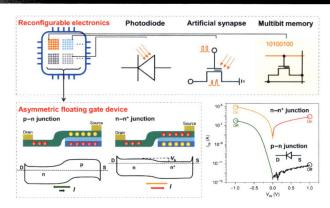
A reconfigurable WSe<sub>2</sub> optoelectronic device is enabled by applying an asymmetric floating gate (AFG) into a flash memory, whose channel can be continuously programmed into p-n or n-n<sup>+</sup> homojunctions by the AFG. As a result, a single AFG device can function as a photodiode, a 2-bit memory, or an artificial synapse under different working modes.
