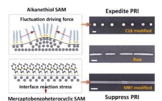
The control on Plateau-Rayleigh instability (PRI) of silver nanowire (AgNW) is readily realized by two kinds of self-assembled monolayers (SAMs), which not only provides the AgNW with superior anti-corrosion but also enables achieving invisible patterning of the AgNW network.
