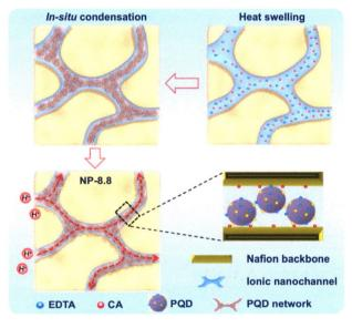
An *in-situ* precise hybridization strategy, mainly containing heat swelling-enabled uniform precursor entrance and microwave-assisted insitu condensation process, is proposed for decorating Nafion ionic nanochannel. This decoration strategy can precisely manipulate the physical topology and chemical environment of ionic nanochannel without affecting the backbone nanophase function.
