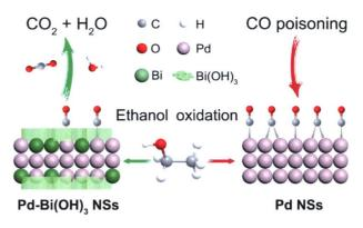
The incorporation of Bi(OH)<sub>3</sub> species effectively tunes the electronic (induce Pd into an electron-rich state) and geometric (separate the Pd ensemble) structures of Pd nanosheets, leading to the improved ethanol oxidation reaction (EOR) activity and superior CO tolerance.
