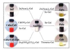
Small molecules in hydrocarbon gels are ideal precursors for synthesizing inorganic nanocrystals.
