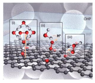
Oxygen functionalization on the hollow mesoporous carbon spheres (HMCSs) results in improved reactivity of these active sites, hydrophilic property of the surface, and tuned adsorption mode of oxygen, leading to significantly reduced overpotential, improved selectivity, and moderate stability for oxygen reduction to H<sub>2</sub>O<sub>2</sub>.
