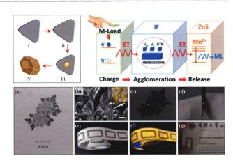
Mechanoluminescence has attracted intensive intentions due to their flexible properties and robust performances for broad applications. However, the development is usually limited in the single-phase materials. We synthesize the heterostructure biphase ZnS:Mn, which delivers efficient mechanoluminescence (ML) due to the abundant defects at the interfaces. The successful applications of ZnS:Mn in ink and papers open its potential in the future.
