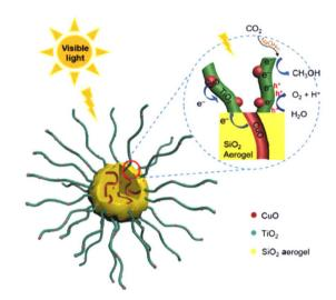
The high crystalline nanofibers and a hierarchical nanocomposite significantly enhanced the density and stability of photoexcited electron-hole pairs. The catalysts combined many advantageous features and exhibited an efficiently photocatalytic reduction of CO<sub>2</sub> without sacrificial agent.
