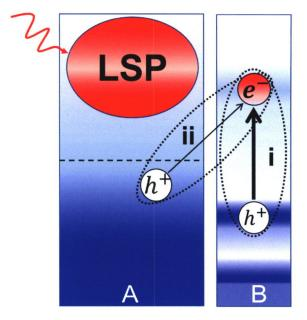
Intramolecular charge transfer induced by localized surface plasmon dominates the plasmon-mediated photolysis of NH<sub>3</sub>, accompanying with a secondary direct charge transfer.
