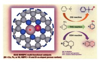
A biomass-assisted pyrolysis-etching-activation (PEA) strategy was developed to construct ISAS metal decorated on N and B co-doped porous carbon (ISAS M/NBPC, M = Co, Fe, or Ni) catalysts with multifunctional features and excellent catalytic activities. They can be used to conduct different types of catalytic reactions, such as O-silylation (OSI), oxidative dehydrogenation (ODH), and transfer hydrogenation (THG).
