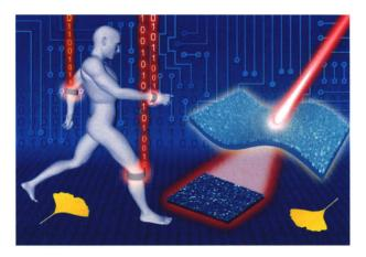
A flexible and stretchable bionic true random number generator (TRNG) is inspired by biological uniqueness and randomness. Random numbers extracted from laser speckle patterns of the flexible TRNG show superior randomness, robustness, and potential in application of flexible networked electronics.
