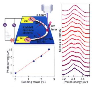
Elastic bending strain induces extraordinary splitting of near band emission and compelling enhancement of ultraviolet photoresponse in GaN nanowires.
