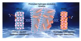
A two-dimensional (2D) layered-nanosheet-on-2D-nonlayered-nanomesh hierarchical heterostructure was fabricated to aim at weakening the strong hydrogen adsorption strength of  $Mo_2C$  by introducing the  $MoS_2$  featuring the strong hydrogen intermediate desorption capacity.
