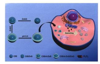
Self-passivation of  $CuInS_2$ -based quantum dots (QDs) is achieved in a simple one-step process, resulting in the spontaneous and rapid formation of ZnO shells outside of  $CuInS_2$ -based QDs. The ZnO shell, serving as a sensing layer, enables sensitive visualization of intracellular hydrogen peroxide generated by mitochondria.
