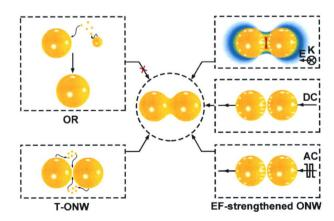
The accomplishment of nanowelding typically requires the input of high energy, possibly causing appreciable damages to the brittle nanomaterial. This study reports an external field (EF, i.e., light, direct current (DC), and alternating current (AC))-strengthened Ostwald nanowelding (ONW) strategy to enable low-temperature nanowelding of Au nanoparticles (NPs) with nanoscale spacing in solution and proposes an electron localization mechanism to understand it.
