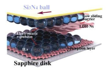
Macroscale superlubricity under ultrahigh contact pressure was enabled by the combination of layered double hydroxide nanosheets with ionic liquid.
