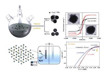
An improved solution pyrolysis route was used to synthesize singlephase cobalt carbides with high coercivity and excellent hydrogen evolution reaction (HER) catalytic activities, in which cobalt nanoparticles (NPs) with different structures were used as raw materials.
