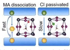
Dissociation of the methylammonium cation in CH<sub>3</sub>NH<sub>3</sub>PbI<sub>3</sub> undermines structural stability, produces deep hole traps, and decreases charge carrier lifetimes. Passivating methylammonium fragments with chlorines restores the stability, eliminates the traps, and makes charge lifetimes even longer than in pristine CH<sub>3</sub>NH<sub>3</sub>PbI<sub>3</sub>.
