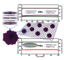
The interlayer-expanded  $VS_2$  nanoflowers via alternated intercalation of N-doped carbon (N-C) monolayers are rationally designed and grown on reduced graphene oxide (rGO). The obtained  $VS_2/N-C@rGO$  nanohybrids, as electrode materials for sodium-ion batteries (SIBs) and potassium-ion batteries (PIBs), exhibit excellent electrochemical energy storage performance.
