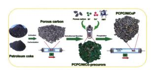
A distinct multifunctional integrated sulfur-host of petroleum cokebased porous carbon/NiCoP composites was prepared for capturing lithium polysulfides (LiPSs) and accelerating the conversion reaction kinetics of LiPSs.
