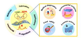
A state-of-the-art review of the flexible Surface-enhanced Raman scattering (SERS) sensors for point-of-care detection was provided from rational design to applications. Strategies of constructing the flexible SERS sensors were investigated in depth, enabling ultrasensitive detection of various analytes and high specificity with a fingerprint-like characteristic.
