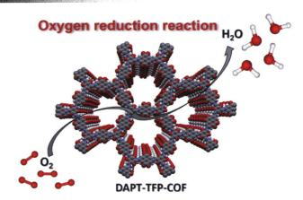
A novel two-dimensional (2D) covalent organic framework (DAPT-TFP-COF) was synthesized by incorporating highly electroactive pyrene-4,5,9,10-tetraone (PTO) units, which was tested as an electrocatalyst towards oxygen reduction reaction.
