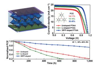
The perovskite solar cells with 35FP-doped have better performance (PCE = 20.45%) compared with undoped device (PCE = 14.11%). The 35FP-doped devices only fell by 20% of its original efficiency after 1, 000 h under ambient conditions without encapsulation.
