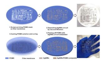
A method was developed for preparing high-resolution, large-size stretchable electrodes by pre-constructing silver nanowires (AgNWs) patterns through screen printing and vacuum filtration then embedding them into a polydimethylsiloxane (PDMS) matrix. These electrodes have been successfully used as a large-size stretchable circuit board for a smart display system and an 18-channel high-density electrode array for surface electromyography (EMG) recording.
