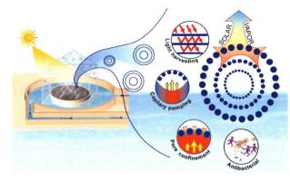
Hollow multishelled structure (HoMS) CuO/Cu<sub>2</sub>O was introduced into the solar-vapour generation. The porous nano/micro HoMS enhanced light absorption, optimized the thermal regulation and water transport, resulting in a high water evaporation rate, and the heterogeneous semiconductors enhanced the production of reactive oxygen species for water disinfection.
