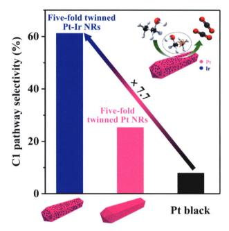
Five-fold twinned (FFT) Pt-Ir nanorods (NRs) are synthesized and exhibit outstanding electrocatalytic performance for ethanol oxidation with a considerable C1 pathway selectivity.
