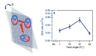
By combing ultrafast spectroscopy and first-principles calculation, we show that the twist angle in transition metal dichalcogenide (TMD) bilayers can act as an effective knob to tune the exciton-exciton annihilation dynamics.
