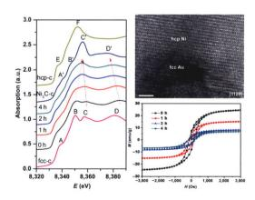
A series of Au@Ni-carbide magnetic materials are achieved from the controlled carbonation of Au@Ni core-shell structures. Hard X-ray absorption spectroscopy (XAS) at the metal K edge and soft XAS at both metal L edge and carbon K edge provide solid evidence for the carbonation process from fcc-Ni (fcc = face centered cubic) to NixC, rather than phase transformation to hcp-Ni (hcp = hexagonal close packed).
