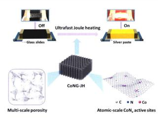
The ultrafast Joule heating process ensures the rapid and stable dispersion of atomic-scale  $CoN_x$  active sites in graphene, while the three-dimensional hierarchically porous architecture promotes the mass transfer efficiency during the catalytic process.
