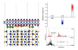
The hydrogenation process can passivate the interface states at the high-k dielectrics, but does not affect the two-dimensional (2D) semiconductors, enabling an improved integration of high-k dielectrics on 2D materials based nanoelectronics.
