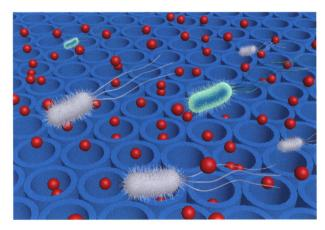
Mesoporous silica coatings (MSCs) with vertical and size-tunable mesochannels are fabricated on a variety of metal substrates via a nanointerfacial oriented assembly approach. Importantly, the MSCs on titanium substrates (Ti@MSCs) exhibit excellent drug adsorption, sustained release, and antibacterial performances.
