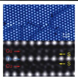
We characterized the structural and electronic modification of 1T-TaS<sub>2</sub> after Cu intercalation. Novel spatial electronic distributions have been identified in different domains, demonstrating the enhancement of interaction between the star of Davids (SDs) due to the interlayer Cu atoms.
