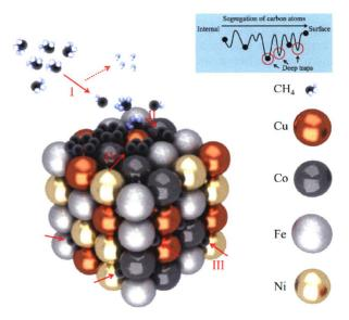
A facile approach to grow few-layer graphene on high-entropy alloy (FeCoNiCu<sub>x</sub>) is presented and the growth mechanism of graphene is systematically investigated.
