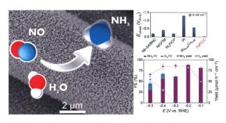
An FeP nanorod array supported on carbon cloth (FeP/CC) behaves as a high-active electrocatalyst with a low onset potential toward NO-to-NH $_3$  conversion, achieving a remarkable Faradaic efficiency of 88.49% and a large yield of 85.62  $\mu mol \cdot h^{-1} \cdot cm^{-2}$  in 0.2 M phosphate-buffered solution.
