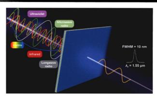
A narrow bandpass filter (NBPF) with ultra-wide stopband based on the coupled Tamm plasmon polaritons (TPPs) transmission theory is proposed and fabricated. It only allows the light with a wavelength of 1.55  $\mu m$  to pass through and shields light with other wavelengths. This performance is much better than the traditional filters and those reported novel metamaterial filters.
