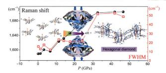
Pressure-induced dehydro-Diels-Alder reaction occurred at  $\sim 7$  GPa. Above 17.0 GPa, the intermolecular sp³ bonding was built up in an amorphous state, that is pressure-induced diamondization. Dehydro-Diels-Alder reaction (decomposition) and diamondization (polymerization) specify the solid-state topochemical reaction, those are scarcely seen in solid-state. The pressure dependence of G band in Raman spectroscopy reflected  $C_{18}Te_3Br_4(Bu-O)_6$  evolution with pressure.
