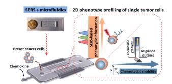
A surface enhanced Raman scattering (SERS)-microfluidic chip has been developed for two-dimensional (2D) profiling of tumor chemotactic and molecular phenotype at single-cell resolution.
