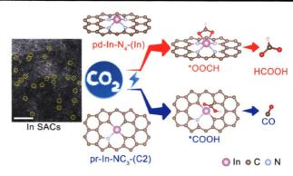
Electrochemical CO<sub>2</sub> reduction (CO<sub>2</sub>RR) selectivity switch from HCOOH to CO in In single-atom catalysts (SACs) enabled by active sites shift from indium center to the indium-adjacent carbon atoms.
