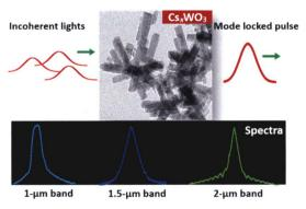
$Cs_xWO_3$  nanorods (NRs) as a novel ultra-broadband nonlinear optical modulator were successfully developed for ultrafast fiber lasers in three key wavelength bands from near-infrared (NIR) to mid-infrared (MIR) region.
