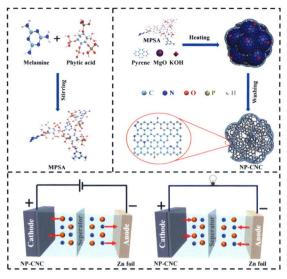
Interconnected N/P co-doped carbon nanocage (NP-CNC) was synthesized from pyrene molecules by using MgO as template and melamine-phytic acid supramolecular aggregate (MPSA) as dopant coupled with KOH activation, presenting outstanding electrochemical properties as electrode material of energy storage devices.
