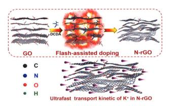
A flash-assisted doping method was proposed to produce nitrogen- and sulfur-doped graphene (N-rGO and S-rGO). Particularly, the assynthesized N-rGO with a high N content of 12.75 at.% and abundant structure defects used as potassium ion battery anodes exhibits ultrafast transport kinetics of K<sup>+</sup>.
