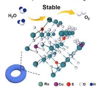
We demonstrate that the incorporation of S into RuCuO nanorings (NRs) can optimize the interaction of Ru and O and significantly suppresses the dissolution of Ru in acidic condition. The optimal catalyst exhibits enhanced stability for 3,000 cycles of cyclic voltammetry test and more than 250 h chronopotentiometry test at 10 mA·cm<sup>-2</sup> in 0.5 M H<sub>2</sub>SO<sub>4</sub>.
