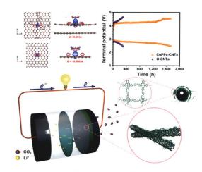
Conjugated copper polyphthalocyanine significantly improved the CO<sub>2</sub> adsorption and carbon nanotubes have excellent electrical conductivity. The composites (CuPPc-CNTs) provide an opportunity for the research of covalent organic polymers (COPs) single-atom catalyst in Li-CO<sub>2</sub> battery field.
