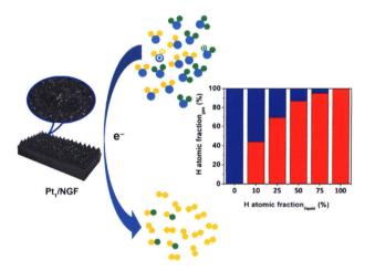
Pt single atom catalysts (SACs) were anchored on nitrogen doped graphite foil by polyol reduction method. The as-prepared Pt SACs exhibited high activity with an overpotential of 0.022 V at 10 mA·cm<sup>-2</sup> toward hydrogen evolution reaction and a high separation factor of 6.83 toward H/D separation.
