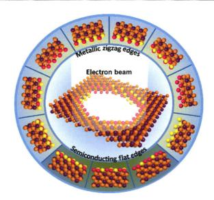
Electron beam irradiation can be utilized to tailor single-layer  ${\rm Bi}_2{\rm Te}_3$  with semiconducting flat edges and metallic zigzag edges with atomic resolution.
