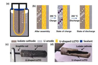
Here, we firstly report a molten Li- $I_2$  battery (MLIB) based on the U-shaped garnet Li<sub>6.4</sub>La<sub>3</sub>Zr<sub>1.4</sub>Ta<sub>0.6</sub>O<sub>12</sub> (LLZTO) ceramic electrolyte tube at a moderate operating temperature of 260 °C, comprised of a molten lithium anode and a molten CsI/LiI eutectic salt cathode. The high active material LiI loading in a single cell can reach up to 593 mg (~ 173.7 mg·cm<sup>-2</sup>).
