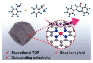
Herein, we report a solid-state transformation strategy to fabricate Co single atom catalysts by introducing Co species from commercial  $\text{Co}_2\text{O}_3$  powders into nitrogen-doped carbon support. Its exceptional catalytic performance in the direct C–C cross-coupling of primary and secondary alcohols was experimentally validated and further confirmed by density functional theory calculations.
