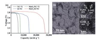
The  $MnO_x/hCNC$  cathode by defect-induced deposition exhibits high full discharge capacity and superior cycle life for  $Li-O_2$  batteries, owing to the boosted reversibility of oxygen reactions by the highly dispersed  $MnO_x$  nanoparticles and the fast charge/mass transfer facilitated by the hierarchical carbon nanocages (hCNC).
