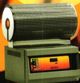
MTF 绕线式管式炉
