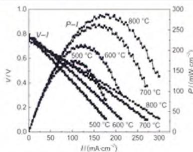
$\text{Pr}_{1-x}\text{Sr}_x\text{NiO}_4$  (PSNO) material with a  $\text{K}_2\text{NiF}_4$ -type structure was prepared by the glycine-nitrate process. The material shows good electrochemical and thermal properties. It is a potential cathode material for use in intermediate-temperature solid oxide fuel cells.
