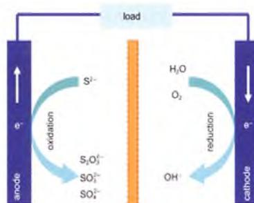
We demonstrate that alkaline sulfide fuel cells containing non-precious carbon-based catalysts can exhibit a considerable power output, while sulfides are deeply oxidized.
