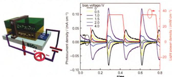
The photocurrent polarity of a bulk heterojunction organic photovoltaic device was investigated and controlled using a ferroelectric thin film.
