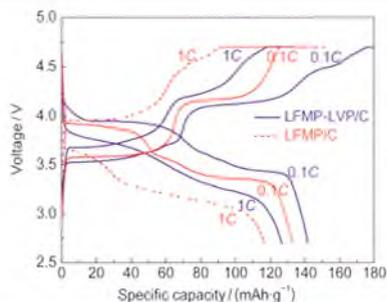
Vanadium modification can be an effective method to improve the electrochemical performance of olivine-type cathode materials.
