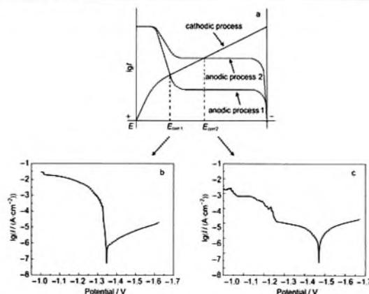
The polarization curve of a micro-arc oxidation (MAO) coating depends on both its main composition and microstructure because of its instability in NaCl solution.
