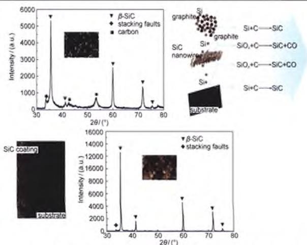
Self-healing pure SiC coating was fabricated and it showed an improved oxidation resistance in C/C composites.
