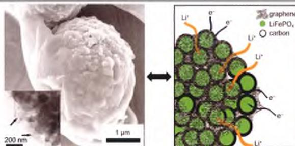
Graphene modified  $\text{LiFePO}_4$  was synthesized by a hydrothermal method and shown to possess excellent electrochemical properties.
