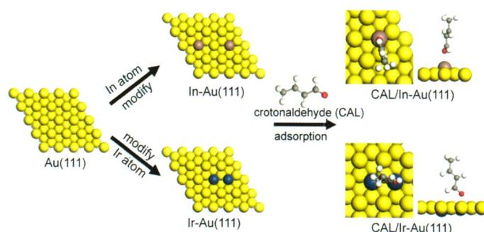
Comparison of Properties of In-Au(111) and Ir-Au(111) Alloy Surfaces, and Their Adsorption to Crotonaldehyde
