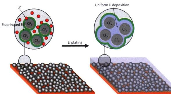
A framework with enriched fluorinated sites enables uniform lithium deposition and stable lithium metal cycling.
