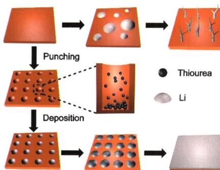
Thiourea acts synergistically with a porous copper foam to guide the growth of lithium in small pores and achieve uniform lithium deposition.
