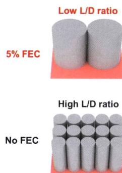
The influence of electrolytes on lithium deposition was quantitatively analyzed, and FEC additive was found to decrease the length/diameter ratio of lithium deposits.
