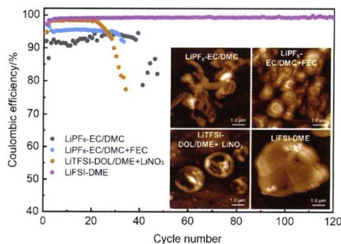
The correlation between the Li plating morphology and Coulombic efficiency indicates that particle-like metallic Li exhibits superior Li plating/stripping reversibility.
