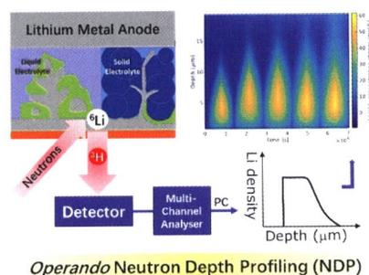
Neutron depth profiling (NDP) is a quantitative and nondestructive technique for the real-time observation of electrochemical behavior of Li in liquid/solid electrolyte-based Li metal batteries.
