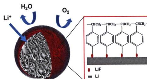
The Li-CNT composite is passivated by a LiF-rich layer through *in situ* polymerization of 4-fluorostyrene.
