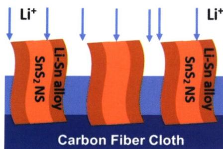
SnS<sub>2</sub> arrays can be converted to Li-Sn alloy and Li<sub>2</sub>S, thereby inducing uniform Li deposition and improving the electrochemical kinetics.
