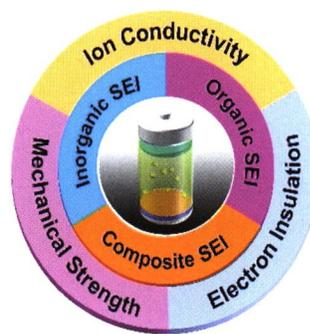
Functional SEIs with the desired ion conductivity, mechanical strength and electron insulation properties are designed to boost the Li anode performance.
