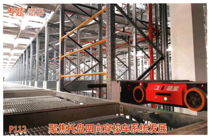
Focusing on the Development of Pallet Four-way Shuttle System
