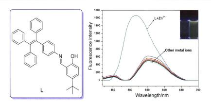
A novel aggregation-induced emission (AIE) effect  $Zn^{2^+}$  fluorescent probe L was constructed with aggregation-induced emission (AIE), tetraphenylethylene as the fluorescent group and 5-*tert*-butyl-2-hydroxybenzene as the recognition group. Its fluorescence properties were studied by UV-vis and fluorescence spectroscopy. The response mechanism of the probe to  $Zn^{2^+}$  was studied by Job's plot, ESI-MS and density functional theory (DFT) theoretical calculation.
