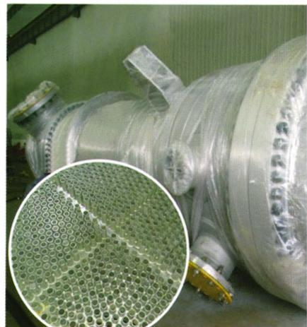
降膜蒸发器(Falling-film evaporator)
