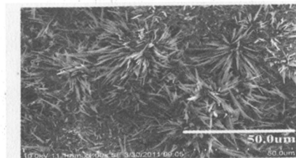
Boric acid has a significant influence on the appearance and morphology of L -Lys·HCl·H 2 O crystals obtained on the self-assembled monolayers of L -cysteine.
