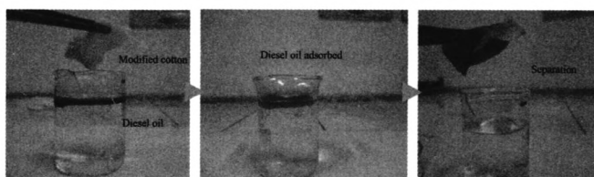
Controllable wetting behavior of the modified cotton and their selective adsorption properties to diesel oil.
