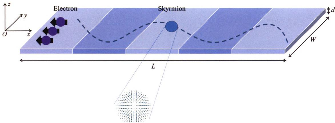
A chiral ferromagnetic film with spatially modulated Dzyaloshinskii–Moriya interaction is placed in the  $x$ - $y$  plane. Spin-polarized electrons are injected to drive the motion of the magnetic skyrmion in the film.  $L$ : Length;  $W$ : Width;  $d$ : Thickness. See: Liping Zhou, Ren Qin, Ya-Qing Zheng, and Yong Wang, Skyrmion Hall effect with spatially modulated Dzyaloshinskii–Moriya interaction, *Front. Phys.* 14(5), 53602 (2019).
