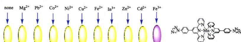
A terpyridine-based Mn(II) complex shows apparent color change upon addition of Fe(III), which can be detected by naked eye.
