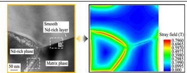
The distribution of the stray field corresponding to the beginning of the reversal process under the applied field approaches zero calculated from the surface in the model, which shows that the largest stray field exists at the intergranular phase. The presence of these non-ferromagnetic phases is expected to produce the magnetic stray field opposite to the spontaneous magnetization in the neighboring grains, thereby reduce the ideal nucleation field
