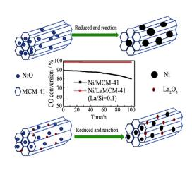
Lanthanum was incorporated via hydrothermal synthesis into a MCM-41 framework structure, the obtained Ni/LaMCM-41 catalyst exhibited excellent catalytic activity and stability for methanation. La reduces the average particle size of the NiO particles inhibits the sintering of the catalyst and the formation of carbon deposits
