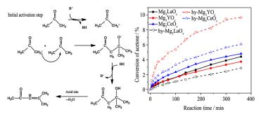
The Mg<sub>3</sub>REO<sub>x</sub> catalysts exhibit a high catalytic activity for aldol condensation of acetone, which is dependent on a homogeneous basic surface of medium strength. Upon hydration pre-treatment, the basic properties on the surface of the Mg<sub>3</sub>REO<sub>x</sub> catalysts were changed markedly, and the hy-Mg<sub>3</sub>YO<sub>x</sub> catalyst has the highest activity
