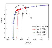
The magnetic properties of the PrFeB magnets with and without GBD. The  $B_r$  was approximately 13.85 kGs, and there were no obvious changes observed. However, the  $H_{ci}$  of the PrFeB magnets with GBD displayed a large increase in different degrees. The smaller orientation direction thickness of the magnet resulted in a larger increase of the  $H_{cj}$ . The comprehensive magnetic properties of the PrFeB magnets is about  $(BH)_{max} + H_{ci} = 74.7$
