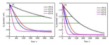
The as-milled alloy shows a much faster dehydriding rate. The time needed by desorbing 2 wt% H2 at 593, 613, 633 and 653 K is 2940, 613, 484 and 185 s respectively for the as-spun alloy, while 848, 355, 232 and 132 s for the as-milled one
