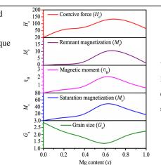
Variation of *D*,  $G_a$ ,  $M_s$ ,  $\eta_B$ ,  $M_t$ ,  $H_c$  with Mg-content for Mg<sub>x</sub>Cd<sub>1-x</sub>Nd<sub>0.03</sub>Fe<sub>1.97</sub>O<sub>4</sub> (*x*=0.0, 0.2, 0.4, 0.6, 0.8 and 1.0) system
