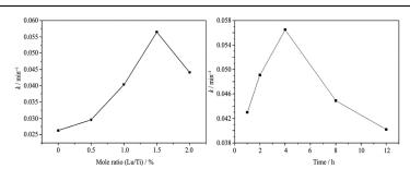
Effects of  $Lu^{3+}$  mole ratio and milling time on photocatalytic degradation reaction rate constants k of MB with  $Lu^{3+}/TiO_2$  as photocatalyst
