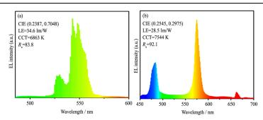
The EL spectra and optical parameters of w-LEDs for NNAO: $0.01Er^{3+}$  (a) and NNAO: $0.03Dy^{3+}$  (b) phosphors under the operation current of 20 mA (recorded at 380 nm excitation)
