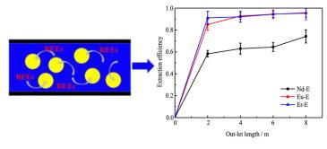
Membrane dispersion mico-extractor was used to recover and enrich the rare earth elements from waste water, the extraction efficiency could be up to almost 100% within 10 s
