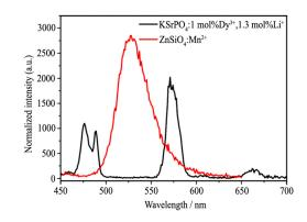
The optimal luminescent sample KSrPO<sub>4</sub>:1 mol%Dy<sup>3+</sup>, 1.3 mol%Li<sup>+</sup> can directly emit warm-white light without two or more luminescent ions co-doped, and its relative luminescent intensity was measured as 60.2% of commercial PDP green phosphor Zn<sub>2</sub>SiO<sub>4</sub>:Mn<sup>2+</sup> under 147 nm excitation
