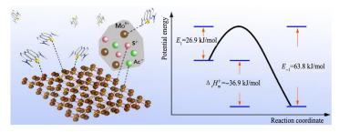
Monoclinic-phase  $Y_2Mo_4O_{15}$  adsorbent with a large adsorption capacity for MB (198 mg/g) were successfully prepared by SSM. Dynamic and thermodynamic properties of the adsorption process are investigated using temperature-dependent adsorption experiments. A possible adsorption mechanism is proposed based on the competitive ion experiments
