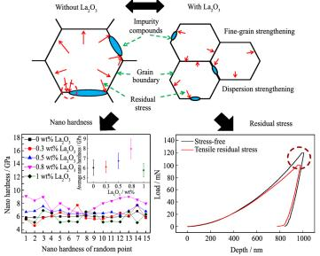
In order to distribute the residual stress in the plasma cladding Stellite 6 coating, the  $La_2O_3$  was added. The results show that the 0.8 wt%  $La_2O_3/$  Stellite 6 coating has the the smallest grain size, the maximum nano indentation hardness and the minimum value of residual stress
