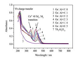
With the increase of the Ga ionic concentration, the diffraction peaks of the 0.5 at%Ce:Yb<sub>3</sub>Al<sub>5-x</sub>Ga<sub>x</sub>O<sub>12</sub> (x =0, 1, 2, 3, 4, 5) garnets exhibited slight shift towards the left, and the main reason causing this phenomena is that the Ga3+ ionic radius is larger than the Al<sup>3+</sup> ionic radius. From the picture, we speculated that the absorption band edge of 250-270 nm was mainly caused by the charge transfer luminescence of Yb3+
