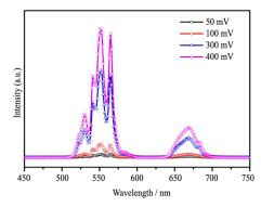
Er-doped PMN-32PT single crystal exhibited upconversion emission properties. The green (531 and 552 nm) and red (670 nm) emission bands were recorded under 980 nm diode laser excitation, corresponding to the transitions of  ${}^4H_{11/2} \rightarrow {}^4I_{15/2}$ ,  ${}^4S_{3/2} \rightarrow {}^4I_{15/2}$  and  ${}^4F_{9/2} \rightarrow {}^4I_{15/2}$  of  $Er^{3+}$ . In addition, the fluorescence intensities of the green and red emissions increased with the excitation power increasing
