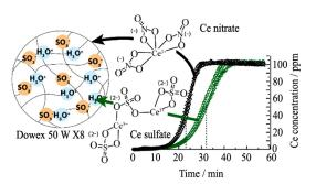
Inductively coupled plasma mass spectrometry Ce<sup>3+</sup> breakthrough curves during Ce nitrate and Ce sulfate sorption on the Dowex 50W 8X
