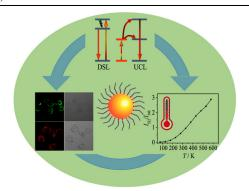
We developed a novel hot-injection method for synthesizing sub-10 nm lanthanide-doped SrFCl nanocrystals with efficient upconverting and downshifting luminescence and demonstrate their potential applications as sensitive luminescent nanoprobes for targeted cancer cell imaging and non-contact thermal sensing
