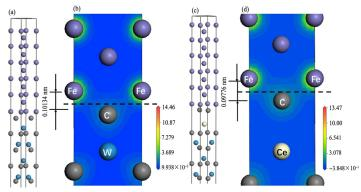
Compared with the un-doped coating interface ( $W_{\rm ad}$ =8.76 J/m²,  $d_0$ =0.10134 nm), the doped coating interface has a smaller interface distance ( $d_0$ =0.09776 nm) and a larger interface binding energy ( $W_{\rm ad}$ =8.98 J/m²). The interface charge distribution shows covalent and ionic bonding at the interface, which indicates that the doped interface is more stable
