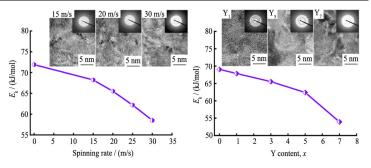
With the increase of spinning rate and Y content, amorphous phase increases and dehydrogenation activation energy decreases
