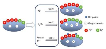
The variation in catalytic performances of Pd/Ce $_{0.67}$ Zr $_{0.33}$ O $_{2}$  catalyst for CO, HC and NO $_{x}$  elimination by the pretreatment atmosphere is revealed
