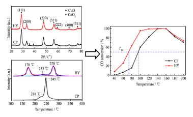
Hydrothermal method prepared  $CuO\text{-}CeO_2\text{-}ZrO_2$  catalyst preserves small crystalline size, high dispersion of active components and high reducibility. Meanwhile, the presence of more CO oxidation sites on the surface and the formation of more  $Cu^+$  species and oxygen vacancies on the copper-ceria interface account for its superior low-temperature activity and  $CO_2$  selectivity, compared with those of the catalyst prepared by coprecipitation
