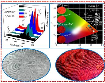
Alkali metal ions ( $M^+ = Na$ , Li, K) co-doped  $ZnAl_2O_4$ : $Eu^{3+}$  (5 mol %) (ZAE) nanopowders (NPs) were prepared via solution combustion route using *mimosa pudica* (MP) leaves extract as a fuel. A 2-fold enhancement in PL intensity was observed in  $Li^+$  co-doped samples. The optimized  $ZnAl_2O_4$ : $Eu^{3+}$  (5 mol%),  $Li^+$  (1 wt%) (ZAEL) NPs wee used to visualize LFPs on various porous, semi-porous and non-porous surfaces through robust powder dusting technique
