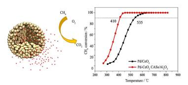
Ordered hybrid  $Pd\text{-}CeO_2$  colloidal assembled spheres (CASs) with highly dispersed Pd clusters were synthesized.  $Pd\text{-}CeO_2$  CASs supported on  $\gamma\text{-}Al_2O_3$  show high catalytic performance and thermal stability in methane combustion. The enhanced catalytic activity can be attributed to the more number of catalytically active Pd-O-Ce sites
