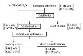
The calcification-leaching of bastnaesite concentrate was studied. Firstly bastnaesite is decomposed by calcification where REs and F are transformed into RE(OH) $_3$  and CaF $_2$ , respectively and both concentrate in calcified residue. Then by HCl leaching, REs and F are separated. In final, 99.2 wt% of fluorine leaves in leaching residue and 72.5 wt% of REs are leached out
