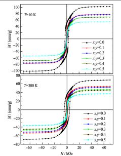
The influence of manganese (Mn) and yttrium (Y) co-substitution on the microstructural, morphological and magnetic properties of strontium nanohexaferrites (Sr<sub>1-x</sub>Mn<sub>x</sub>Fe<sub>12-y</sub>Y<sub>y</sub>O19;  $0.0 \le x=y \le 0.5$ ) was examined. The magnetic hysteresis loops of the various produced nanohexaferrites indicate ferrimagnetic behavior
