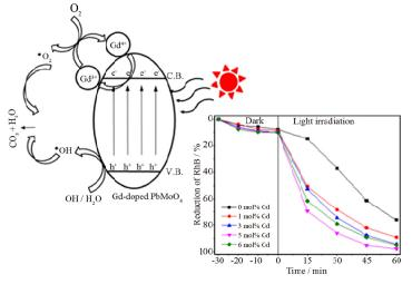
Schematic illustration for photocatalytic mechanism of Gd-doped PbMoO $_4$  nanoparticles and reduction of RhB in the dark and under UV radiation caused by 0 mol%, 1 mol%, 3 mol%, 5 mol% and 6 mol% Gd-doped PbMoO $_4$  nanoparticles
