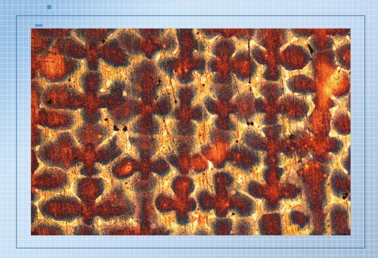
Effect of nitrogen on micro-pores in DD33 single crystal superalloy during solidification and homogenization
