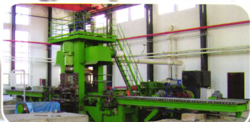
650冷热两用四/六辊板带轧制中试线
